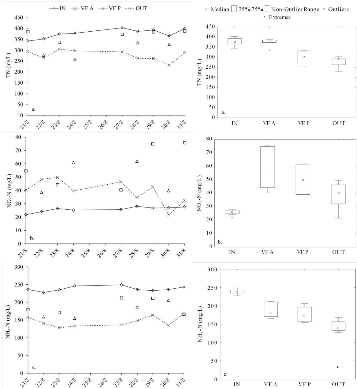
Figure 2. Time patterns and box and whiskers plots of the nitrogen forms during the sampling period: TN(a.); NO<sub>3</sub>-N (b.) and NH<sub>4</sub>-N (c.).
